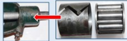
Bearing shell A-8535 and roller bearing A-8530-A which sits inside the casting at front.
