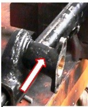
The 7 tooth sector housing is part of the box and cannot be removed.
