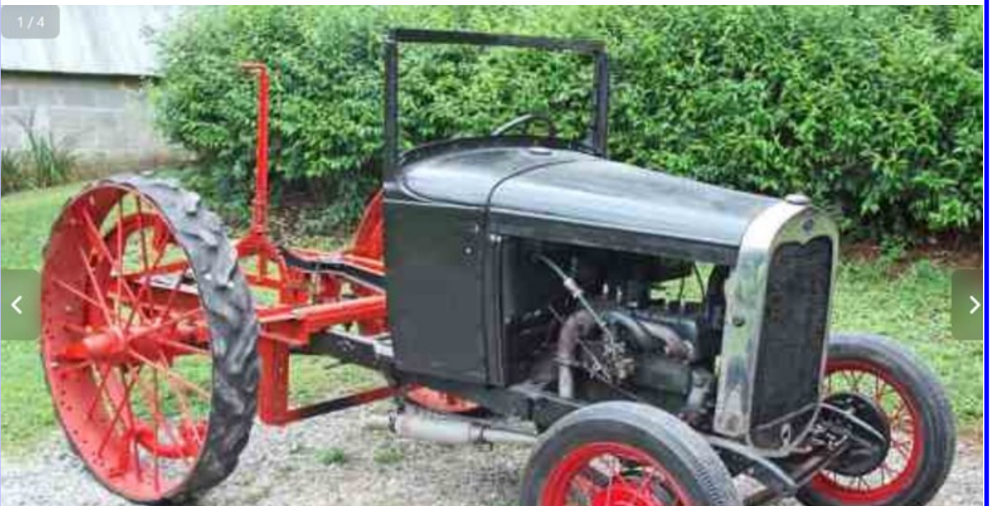
Ronnie Kitts installed a restored conversion kit on his 1930 Ford Model A, creating a crossover between his hobbies: vintage Fords and vintage tractors.
