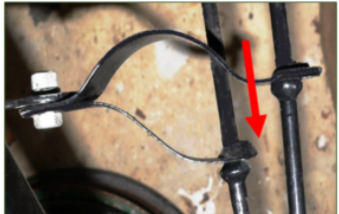
This shows the rear flat spring brake rod anti rattlers pushing the brakes off.
