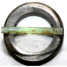
Gauge glass showing thickness of 3/32" x 1 1/8"
