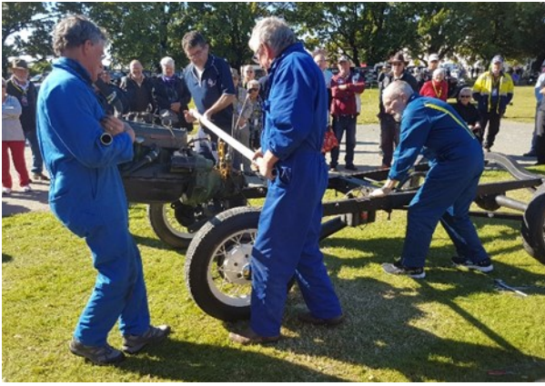
Pulling apart and putting back together a Model A chassis.
