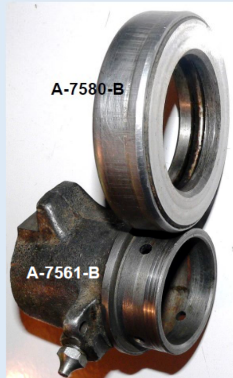
Clutch thrust bearing positioned on the clutch thrust bearing hub.
