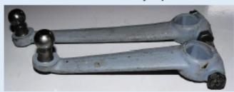
Always secure the arm to the shock absorber shaft very firmly and pin. I have seen a few shocks where the arms had never been removed. Now for the real purists only, when the pin was inserted through the mounting bolt castellated nut, only half of the pin was bent back. The other half of the pin was left straight.
