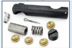
Originally all linkages were tubular. That's what we are discussing here. To install the linkage components to the shock arm and to the perch bolt ball can be tricky. The internal parts have to go in the right order. Pictured right. Start at the bottom. Add a brass cup to the bottom of the linkage with grease. Insert the perch bolt ball and then another cup. Then the spacer, cup, shock arm ball, cup and the threaded top cap. All this
