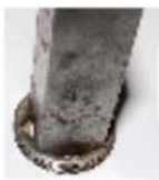
1" square bar is ideal to remove the inner ring.
