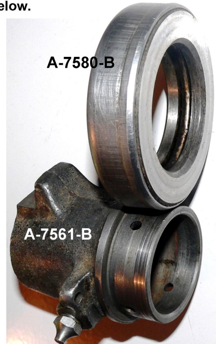
Clutch thrust bearing positioned on the clutch thrust bearing hub.
