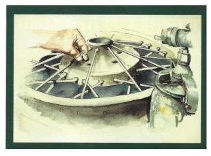
wheel turns. Voila! There goes a wheel making a nice dent in the fender, a squared off backing plate and brake drum, plus other damage to the occupants of your car and any other object it may hit. A good choice is to block the lug nut holes with old lug nuts set in place while painting. This protects the holes and makes for a better tighter holding hole.
