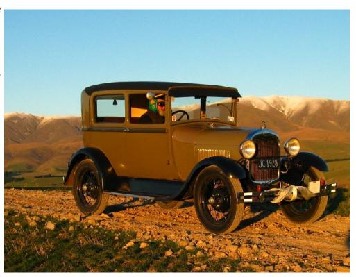
There have been a couple of minor refinements to improve the experience of the Irishman's Rally which can always be put back to original if required. Modern shocks, and webbing in the front seats instead of the springs, blinkers and oversized handmade wheel nuts.
